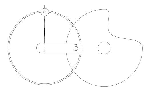
Align the hour hand and minute with the twelve o'clock direction and press them into the central shaft
