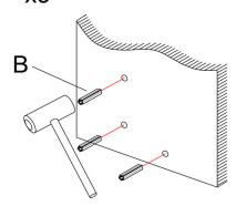
Step 3: Plug the expansion rubber cap into the hole.
