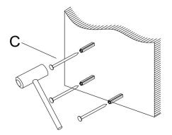
Step 4: Nail the screw into the expanded rubber cap, with the nail head reserved for 5mm, and hang the product back hook on the screw to finish.
