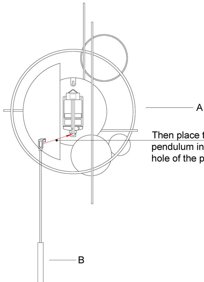
Then place the clock pendulum in the hanging hole of the pendulum.
