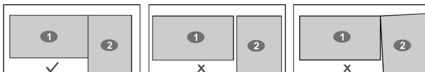
·Holes on the bars and poles are not aligned, so screws can't be installed.
