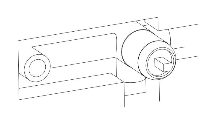
3. The installation in the wall is completed and the switch is opened for sealing test.
