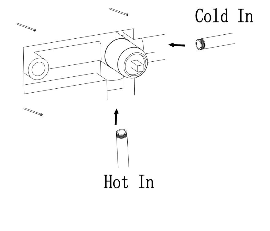
2. Turn off the main switch, adjust the cold and hot water inlet interface and the upper and lower water outlet interface, and use screws to fix the value body in the wall.
