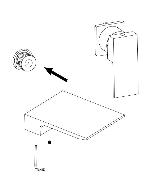
6. Install the spout part: use the connecting pipe to connect the left outlet of the value body to the interface of the spout.
