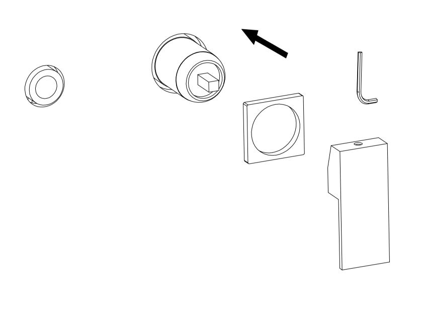
4. Install handle: put two handles on top and lock with hexagonal wrench.
