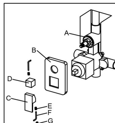
3. Remove the protective cover when the finished wall is completed and install the escutcheon (B) to the valve (A) and press it against the finished wall. Then, install the handle (C) and diverter knob (D), tighten set screws (E) with Allen key (F), and put on the indication buttons (G).
