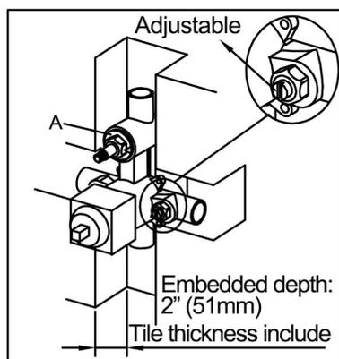
1. Fix the shower valve (A) into the wall. Use a level to ensure that the valve is straight and level. The distance between the bottom of the body and the surface of the tile is 2" (51mm).
