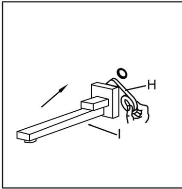
4. Turn the water on for 1 minute to flush any debris. Apply Teflon tape (H) to the threaded tail pipe and install the tub spout (I) into the outlet on the wall.
