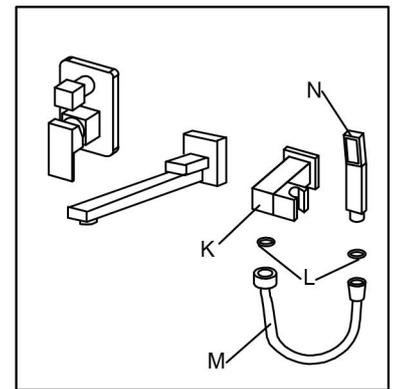
6. Add rubber washers (L) at both ends of the shower hose (M). Connect shower hose (M) to the wall supply holder (K) and hand shower (N). Then, place the hand shower (N) to the wall supply holder (K).
