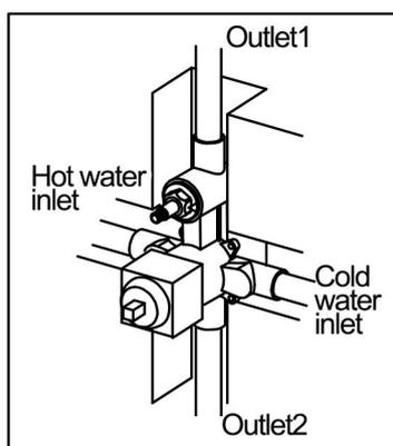
2. Wrap Teflon tape around the pipe threads and connect hot and cold water supply lines and in-wall pipes (not included) as desired to the valve. Turn on the water supply and open the cartridge to check for leakage. Then, put on the protective cover.
