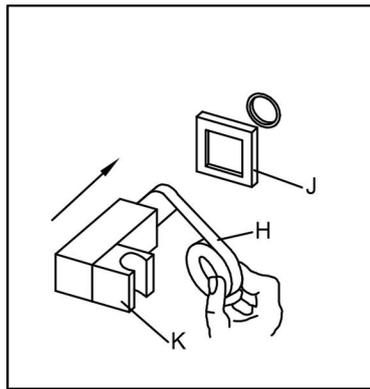
5. Apply Teflon tape (H) to the threaded end, then fix the cover plate (J) onto the wall supply holder (K) and screw the wall supply holder (K) into the hand shower outlet.
