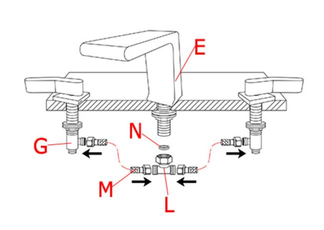
5. Install the triple tube (L) by screwing onto the threaded tail pipe of the spout body (E). Make sure to add the rubber washer (N) inside of the female end of the triple tube (L). Screw waterlines (M) into the triple tube (L) and the
