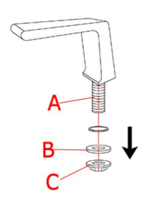
Remove rubber washer (B) and mounting nut (C) from the threaded pipe (A).
