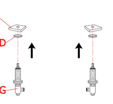
3. Remove O-ring (D) and base plate (F) from the valve (G).
