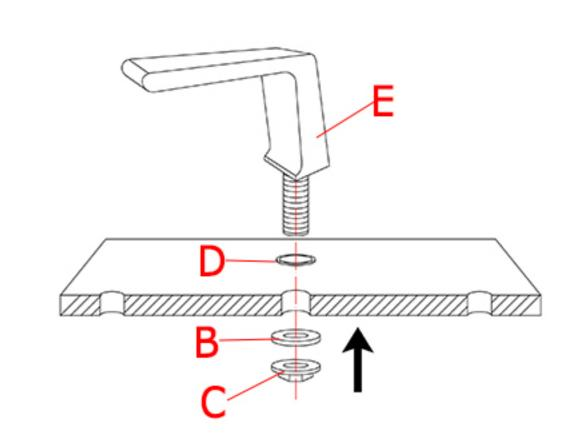
2. Fit the O-ring (D) into the bottom groove of the spout body (E). Insert spout body (E) into the specified drilled hole on the countertop. Install rubber washer (B), mounting nut (C) onto the threaded tail pipe underneath the countertop. Adjust the spout body (E) correctly and secure with mounting nut (C) tightly.
