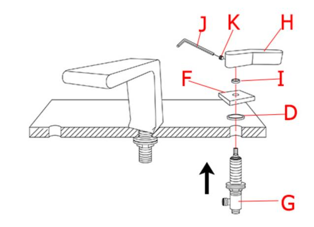
4. Install valve (G) into the specified drill hole underneath the countertop. Fit the O-ring (D) into the base plate (F). Place base plate (F) and fit the washer (I) to the valve (G). Then, screw the handle (H) into the valve (G) and tighten set screw (K) with Allen key (J).
