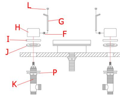
4. Install valve (K) into specified drill hole underneath the counter top. Fit the foam washer (J) into the base plate (I) and screw the base plate (I) and handle (H) into valve (K). Adjust the height and position of valve (K), then screw mounting nut (P) to tighten valve (K) underneath counter top securely. Tighten set screw (F) with Allen key (G) to fix the handle (H) and then place indication button (L) on handle (H).
