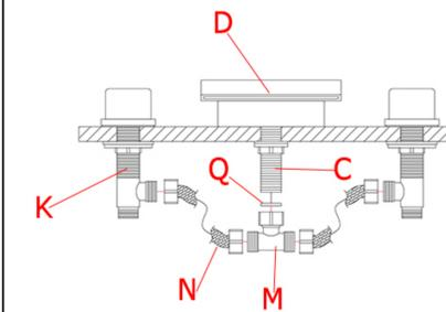
5. Install the triple tube (M) by screwing onto the threaded tail pipe (C) of the spout body (D). Make sure to add the rubber washer (Q) inside of the female end of the triple tube (M). Then, screw waterlines (N) into triple tube (M) and valve (K) according to the picture.
