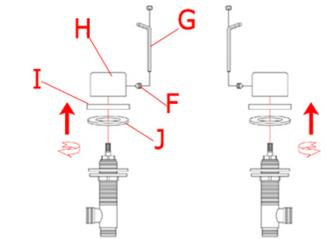
3. Loosen the set screw (F) with Allen key (G) and remove handle (H), base plate (I) and foam washer (J).
