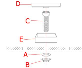
2. Screw the threaded pipe (C) to the spout body (D) through the decorative base (E) and insert spout body into the specified drill hole on the countertop. Install rubber washer (A) to the threaded pipe (C) from underneath the counter top and then screw the mounting nut (B).
