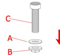
1. Remove the rubber washer (A) and mounting nut (B) from the threaded pipe (C).
