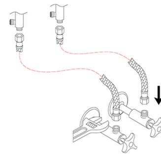
6. Connect waterlines (**not included**) onto the bottom of valve and then to main water supply line.
