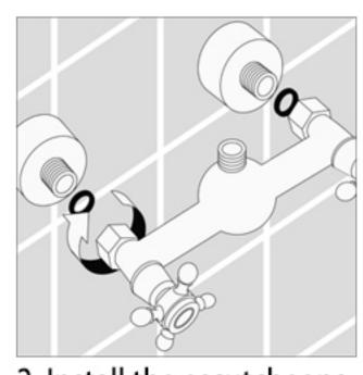
2. Install the escutcheons. Fix the washers into the inlets on the valve body. Install the connecting threads on the s-unions.
