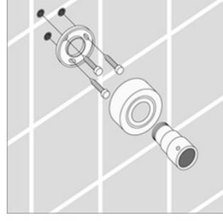
3. Drill the holes and install the anchors. Fix the mounting plate to wall with screws.
