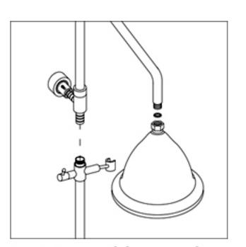
4. Put on rubber washer and thread the showerhead into the shower arm. Screw the riser into the shower arm assembly. Then, locate the shower arm assembly into the mounting bracket and tighten the screw with a screwdriver.
