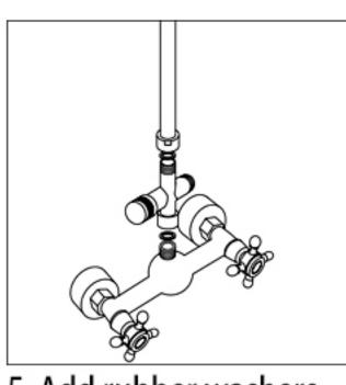
5. Add rubber washers to both ends of diverter and screw diverter into the valve outlet. Then level and fix the riser securely over the diverter outlet.
