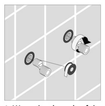
1. Wrap the threads of the s-union with teflon tape. Screw the s-unions into the female fittings of water supplies. Make sure that the s-unions are level.
