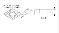
1.N-box in-wall depth:D≤46mm, N-box more than 2mm of tiles.
