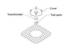
5. Take spare parts, cover, test parts and gradiometer.
