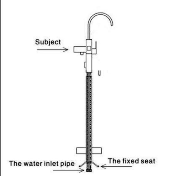
3. Install the flexible hose now and ensure the flexible hoses are hand tightened into place (DO NOT USE SPANNER TO TIGHTEN AS IT CAN DAMAGE THE O-RING). The flexible hoses are to be fitted into the correct inlets for hot water and for cold water.
