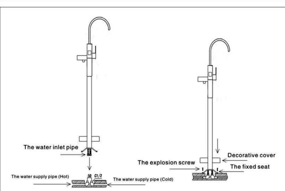
Connect another side of the flexible hose to the water supply pipe. Make sure they are to be fitted into the correct outlets for hot water and cold water. 6. Use the explosion screw to fix the base on the ground, and put the base cover over the base.
