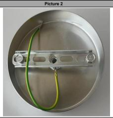
Step 1: Remove the accessories on the hanging plate preinstalled on the top of the suction top plate; Fix the hole position on the ceiling with the hanging plate, and fix the hanging plate on the ceiling with screw G after drilling the hole.
