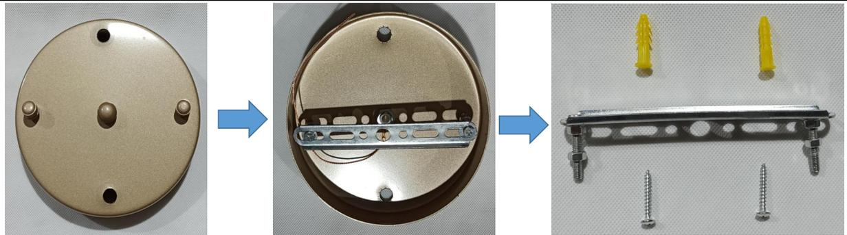
Step 1: Remove the hanging plate from the ceiling plate C first, and then fix the hanging plate on the ceiling with rubber plug H and self-tapping screws I.
