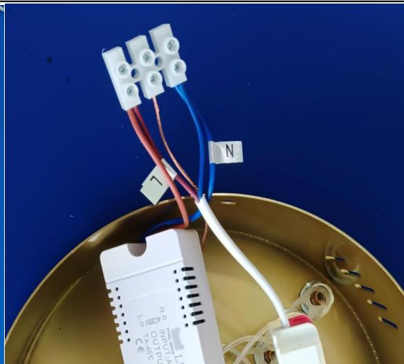
Step 2: As shown in the picture, connect the zero line(blue), the fire line (red), and the ground line(bare copper color) to the terminal, and then connect the corresponding home power supply.
