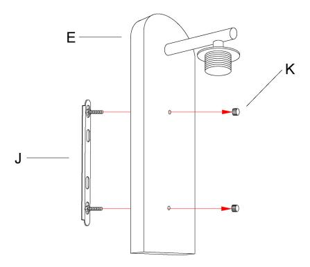
Remove the pre-installed nut first
