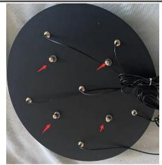
Step 3: Fix the top plate with screw F.
