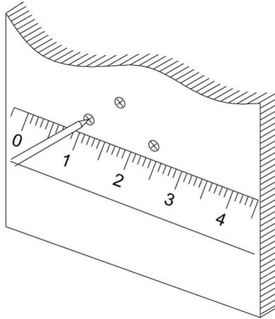
Step 1: Select the location of the wall space to be installed. Measure the distance of the product hook with a ruler, measure the same distance on the wall (if the product has only one hanging hole, you can skip this step), and mark the hole position on the wall with a pen.
