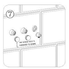
WHEN THE TILE IS IN PLACE, USING SCREW TO FIX HANDLES AND TIGHTING THE SHOWER HOLDER WITH RAW TAPE.
