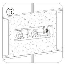
DOUBLE CHECK PIPE CONNECTION, NO LEAKING IN WATER TEST AND OTHER CONCEAL PARTS ARE INSTALLED FINISHED. THEN, CONCEAL BOX AND PIPES ARE SEALED AND FIEXD WITH FILLER.
