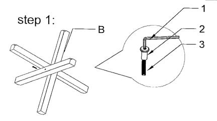
Connect Stainless steel pillar (B) by Screw (E) (M8\*80),tighter, one by one
