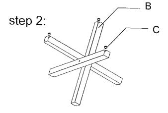
Install the round aluminum cake (C) on the stainless steel pillar (B)as shown.
