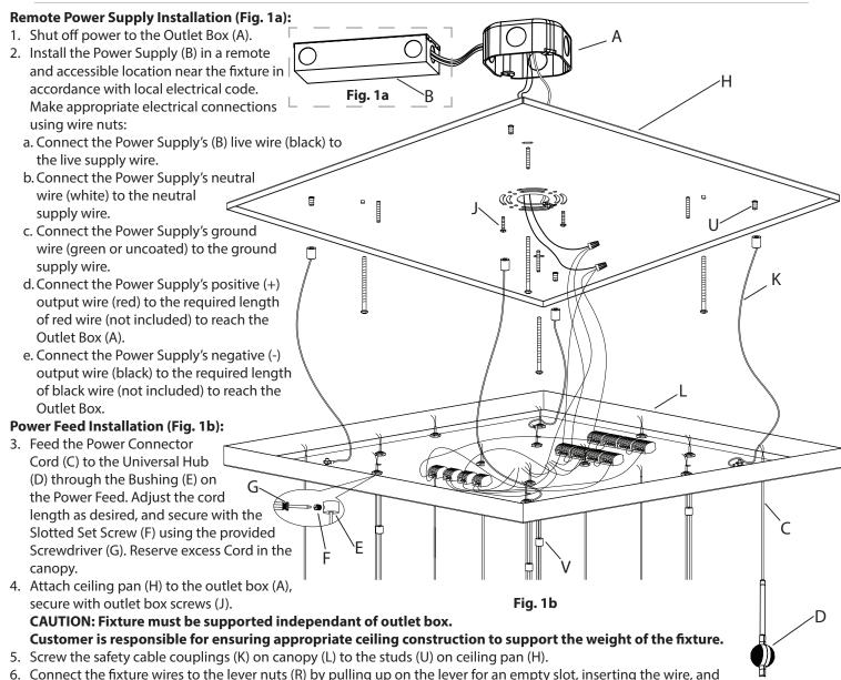
pushing the lever back down to lock. The white inner conductor (S) and black outer conductor (T) on each cord (C) must be
